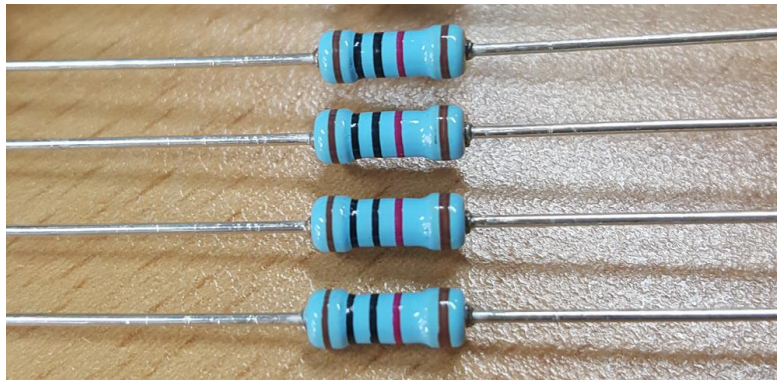
(Figure) 1% tolerance metal film resistor
