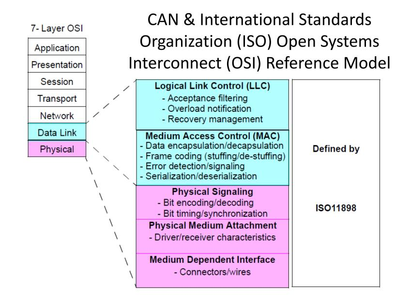
High level CAN Protocols implement Application layer and skip the four intervening layers
