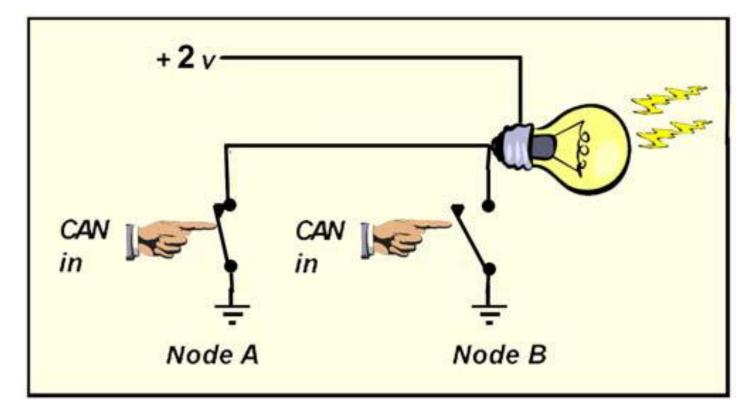
Closing Node A switch **OR** closing Node B switch turns on the light.
