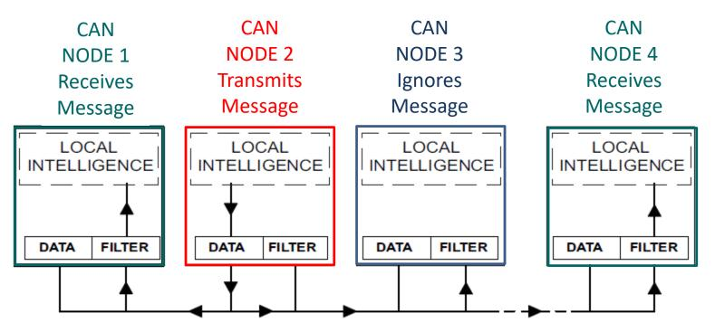
One node transmits, all nodes listen and processor data frames selectively. Message filtering is typically performed in transceiver hardware. This data flow supports a broad range of network communication models:
