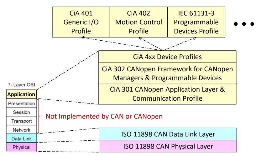
High level CAN Protocols implement Application layers and skip the four intervening layers
