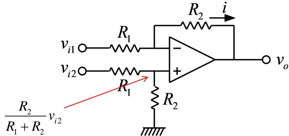
$$i = \frac{1}{R_1} \left( v_{i1} - \frac{R_2}{R_1 + R_2} v_{i2} \right)$$
