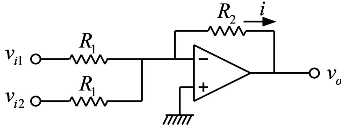
$$i = \frac{v_{i1}}{R_1} + \frac{v_{i2}}{R_1}$$
