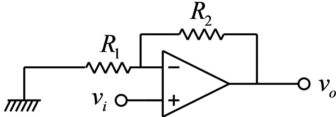
$$v_i = \frac{R_1}{R_1 + R_2} v_o$$
