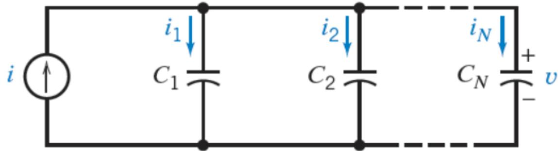
$$C_p = C_1 + C_2 + C_3 + \cdots + C_N = \sum_{n=1}^N C_n$$
